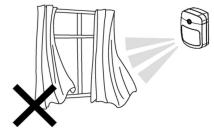
Avoid installing the PIR in areas where machines such as air conditioners or heaters may cause rapid change in temperature in the detection area.
