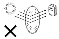
Avoid reflecting surface in the detection area. Reflected infrared signatures may lead to false alarm.
